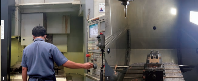
1. From left, Kanagata Factory Manager Kittipong Sonsai and OSG Thai Sales Representative Tantip Luangthongsri. 2. Kanagata Factory Manager Kittipong Sonsai. 3. Kanagata's operator prepares for the machining of a mold. 4. OSG's AE-BD-H carbide ball end mill and a high-hardness steel mold.
