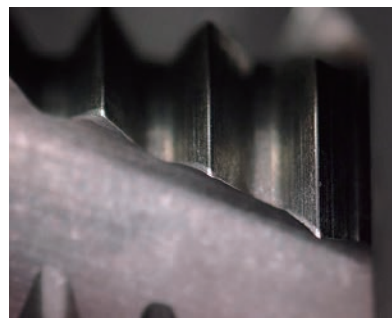
No.1 (after cutting 8,800 threads)
