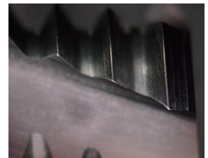
No.2 (after cutting 8,800 threads)
