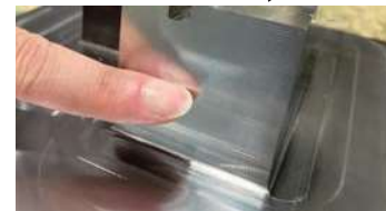
Finished surface by PFB-BR
